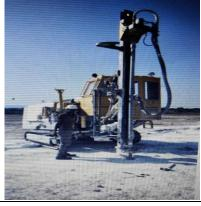
Drilling with water injection
