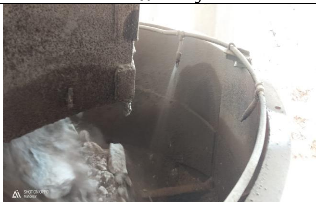
Water fogging System arrangement at Cone
