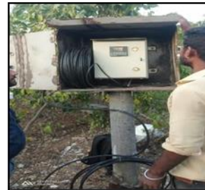
A Visual of Digital Water meter, Digital water level recorder along with telemetry service.
